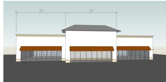
*This diagram illustrates the disruption of horizontal planes at least every 25 feet through the use of a change in plane and the use of a tower.*
